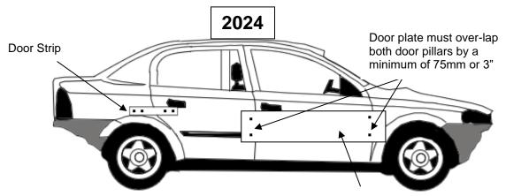
The Door plate must be fixed by either four 16mm or 19mm bolts or studs, or six 13 mm bolts or studs, through both the door pillars. No slotted holes allowed
